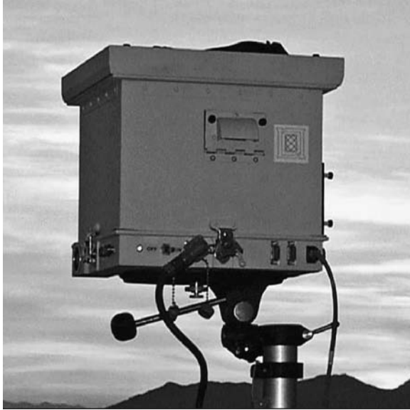
FIGURE 1.25 Prototype biological agent warning sensor.
